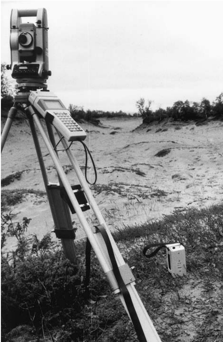
Fig. 2. The levelling equipment (tachymeter and datalogger) at the benchmark at Petsimjärvi dune field. View towards the north. Notice the elongated form of the blowout and the steep slopes at the secondary rim deposits at the edges. Vascular plants Empetrum nigrum and Arctostaphylos uva-ursi support small sand hummocks
