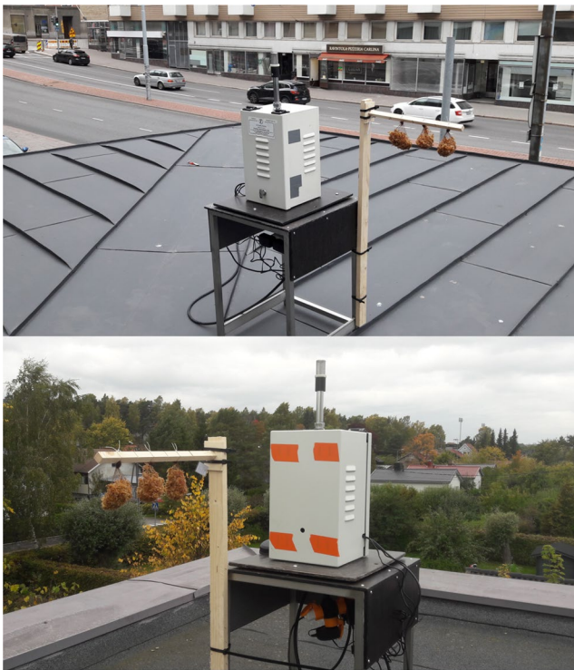
Fig. 2 Osiris monitoring sensors and moss bag sample collectors at Aninkaistenkatu (above) and at Vasaramäki (below)
