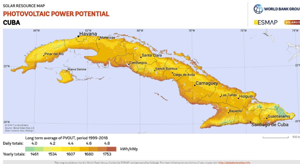
Fig. 1. Cuba, photovoltaic power potential, 2026 [5]. Provided under CC BY 4.0 license.
