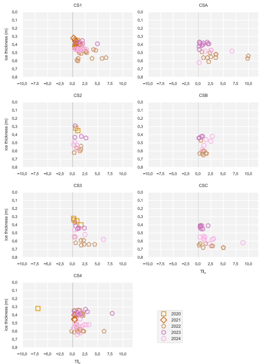
Figure 13. Streamwise turbulence intensity, TI_u , and ice thickness across cross-sections. Each point represents an ADV measurement, color-coded by year.
