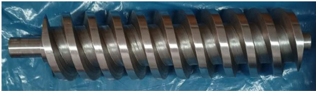
FIGURE 4 | The AISI 1020 steel rotor with trapezoidal thread.
