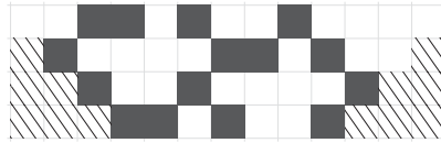
FIGURE 11. Moving a 1101001 one step to the right.
