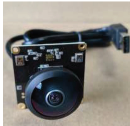
Fig. 6: PICAM360 camera module (Picam360 Developer Community, P. I 2023). USB-a connector allows for an easy integration with Laykka platform.
