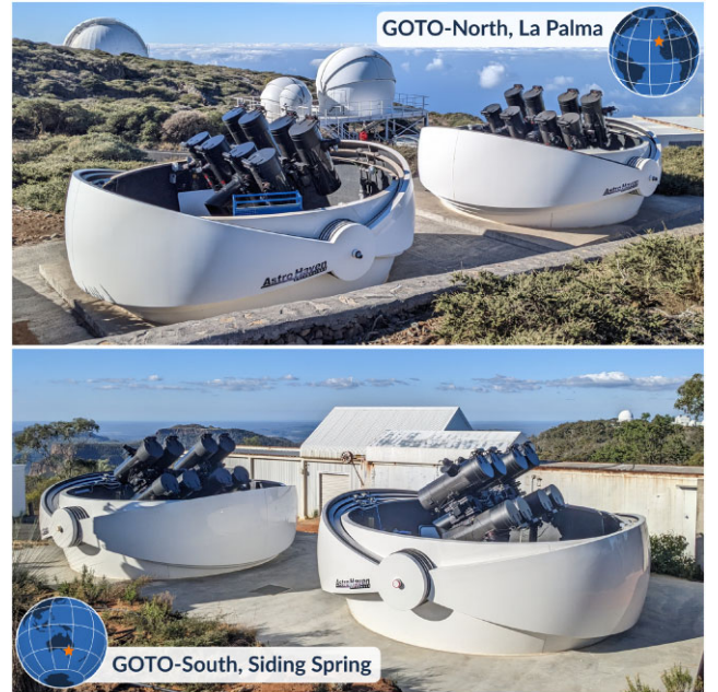
Figure 1. The full configuration of the GOTO telescope network in April 2023, comprising 32 robotic unit telescopes distributed across four domes, two domes at each of the two sites. Top: GOTO-N, located at the Observatorio del Roque de los Muchachos on La Palma, comprising GOTO-1 (left) and GOTO-2 (right). Bottom: GOTO-S, hosted at Siding Spring Observatory in Australia, consisting of GOTO-3 (left) and GOTO-4 (right). Figure credit: M. J. Dyer et al. 2024.
