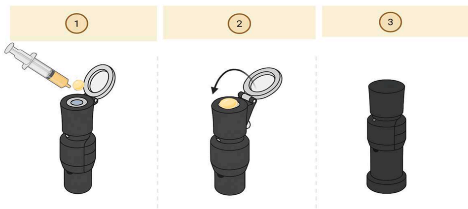
Fig. 1. Sample preparation for near-infrared (NIR) spectroscopic analysis using drop-on-window technique: Step 1: A small amount of semi-solid formulation is dispensed onto the measurement window of the NIR sample holder using a syringe. Step 2: The holder is closed to ensure uniform sample spreading across the window. Step 3: The sample is inserted into the NIR spectrometer for spectral data acquisition. This method enables non-destructive, contact-free analysis of semi-solid materials.
