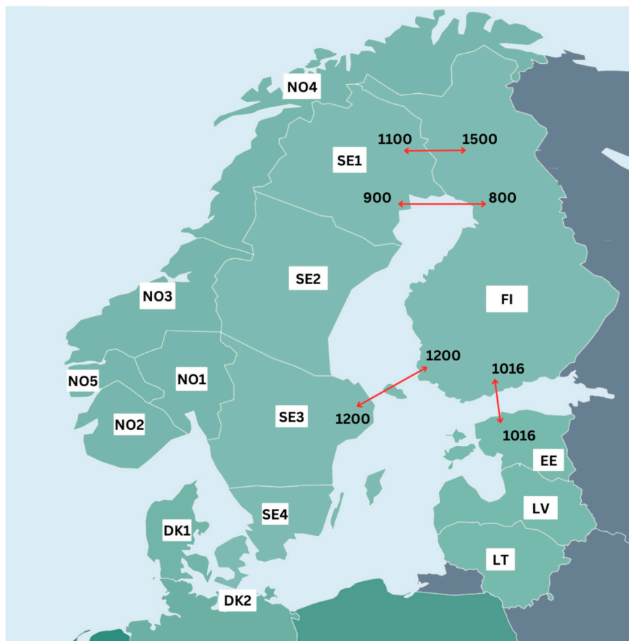
Fig. 2. The Nordic and Baltic Bidding Zones of the Nordpool electricity market, which are modelled in detail in this study [51]. Transfer capacities for Finland are shown as Net Transfer Capacities (NTC).
