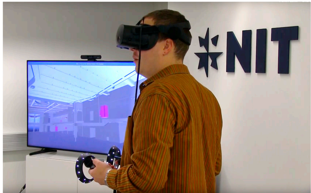
Figure 4. A user viewing a 3D model of a ship interior, wearing a HP Reverb G2 head-mounted display and hand controllers.
