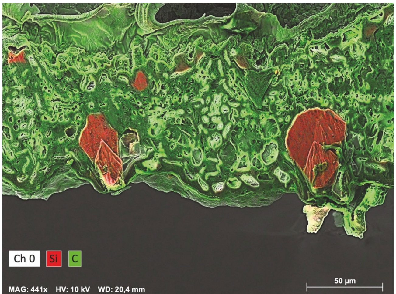
Fig. 2. SEM–EDS micrograph of a leaf where phytoliths (red) are located in the upper side of the leaf. The distance between phytolith particles is 120 \mu\text{m} . Original magnification 441 \times , bar = 50 \mu\text{m} ).
