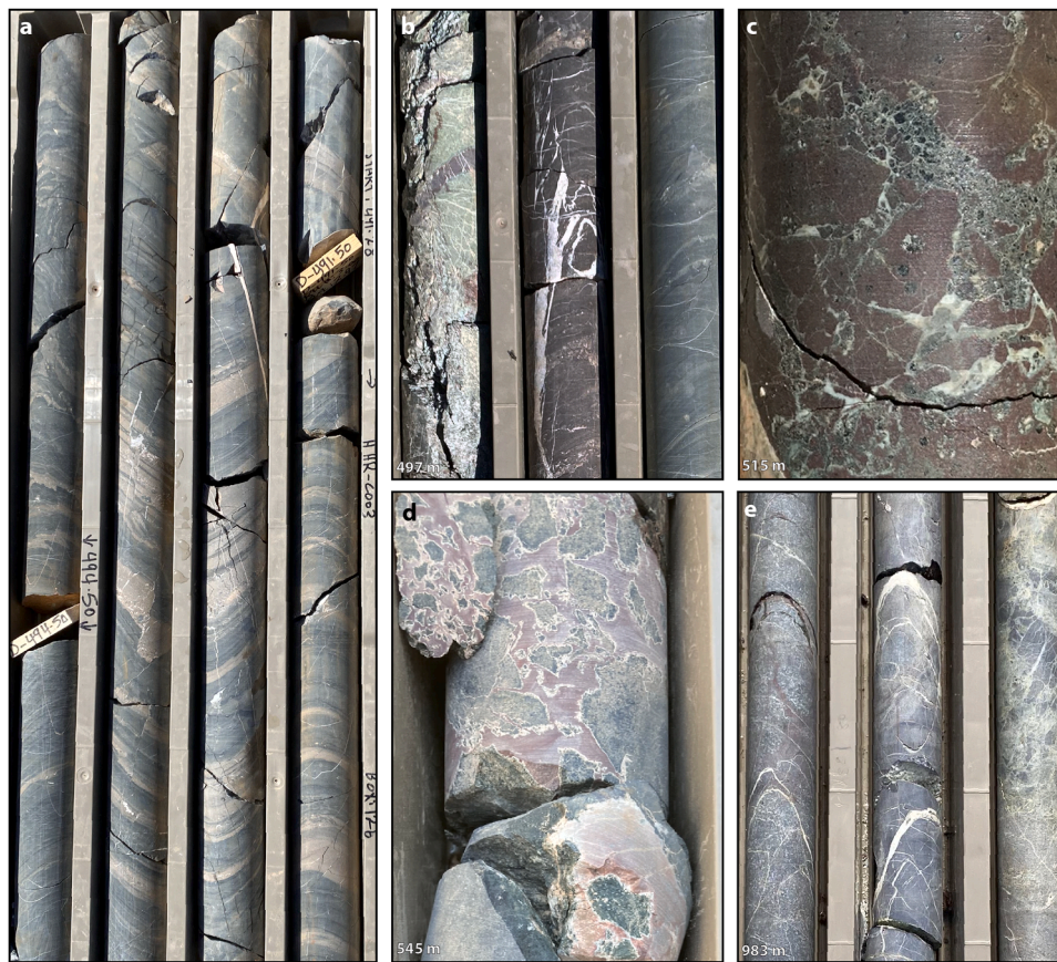
Fig. 6. Drill core photographs of the wells HHR-C002 and HHR-C003. (a and b) Laminated mudstone transected by multiple small displacement faults and veins. (c) common cataclastic texture associated with veining and polyhedral fractures, typical of rocks that have experienced hydraulic brecciation. (d) Cataclastic texture and veining associated with precipitation of rhodonite-rhodochrosite, typical of rocks affected by high-temperature ( \sim 300 °C) hydrothermal fluids. (e) Proterozoic basement rock displaying intense cataclastic texture, polyhedral fractures, and transected by multiple calcite and milky quartz veins. Drill core lengths are one meter for the entire length of the box and a diameter of four cm.
