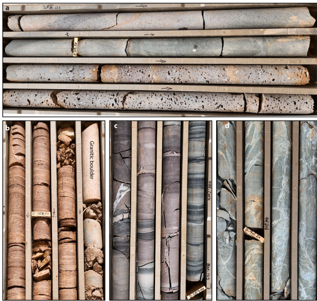
Fig. 7. Drillcore photographs of the well HHR-C004. (a) Massive and vesicular lavas of the Rahat. (b) Gravel up to boulder size overlaying sub-horizontal red laminated mudstones presumably of Miocene age. (c) Sub-horizontal laminated mudstones interbedded with very fine-grained sandstone likely deposited during the Cenozoic. (d) Proterozoic basement rocks with pervasive calcite and milky quartz veining. Drill core lengths are one meter for the entire length of the box and a diameter of four cm.
