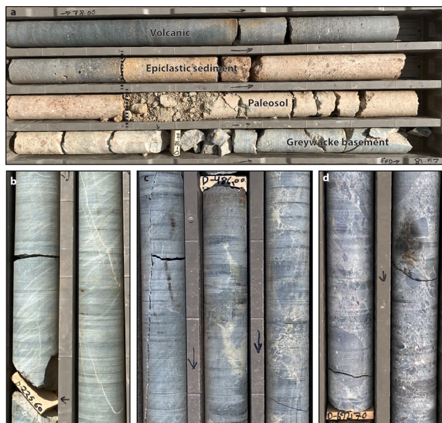
Fig. 5. Drill core photographs of the well HHR-C001. (a) shows the contact between the Rahat lavas and the Proterozoic basement. (b) Typically, massive metasedimentary (greywacke) rock of the Neoproterozoic basement transected by multiple calcite veins. (c) Massive greywacke with pervasive calcite cementation and polyhedral fracturing typical of hydraulic brecciation. (d) Massive metaconglomerate with pervasive calcite cementation. Both greywacke and metaconglomerate rocks do not show visible porosity. Drill core lengths are one meter for the entire length of the box and a diameter of four cm.
