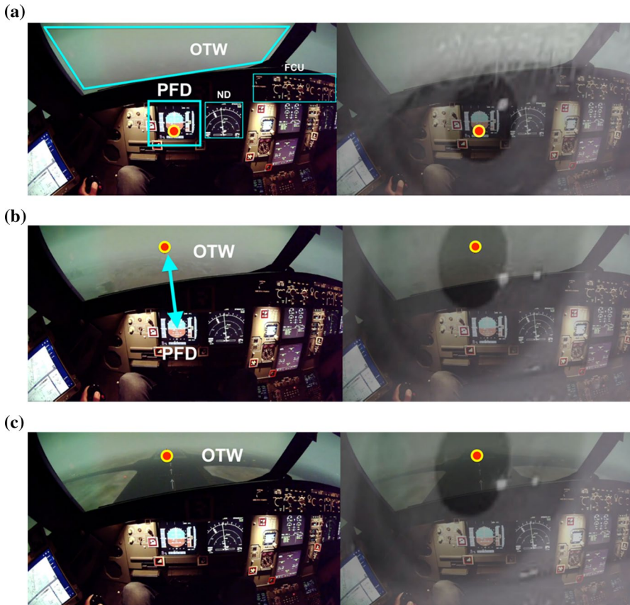
Fig. 3 a In the first stage, after the first callout ‘Hundred above,’ the PF should primarily monitor the PFD. b In the second stage, after the callout ‘Approach lights,’ the PF should switch attention between the PFD and OTW. c In the third stage, after the callout ‘One hundred’, the PF should only be looking at the OTW
