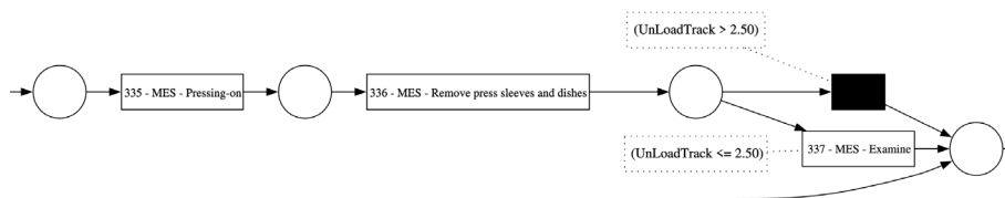
Figure 3: Example of an annotated decision point for an optional examination step in the Petri net for the most common wheelset type
