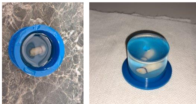
Figure 3. The embedded composite-filled samples in epoxy.
