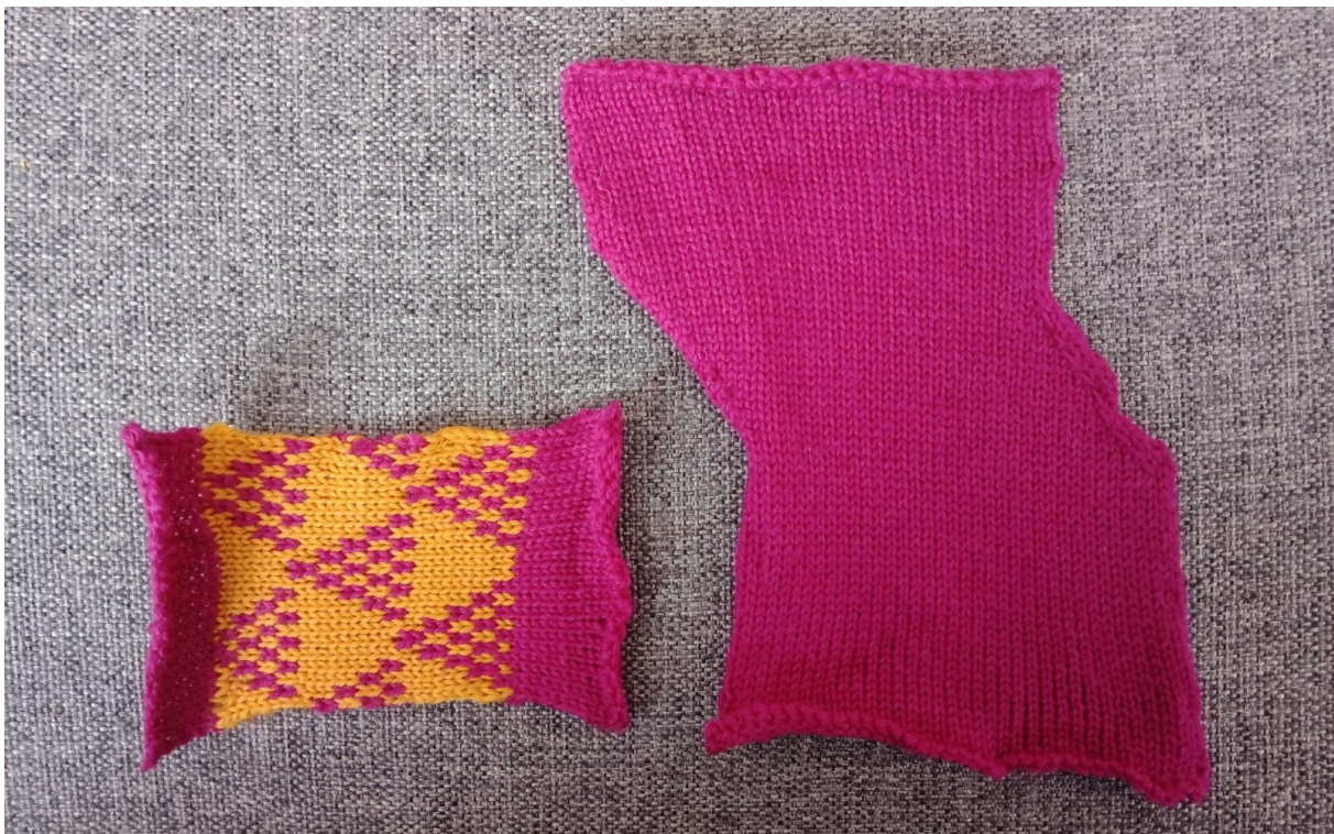
FIGURE 3. Multi-coloured and flat single knit with decrease and cast on exercises with machine. Photo source and courtesy: Course 2: 10.
