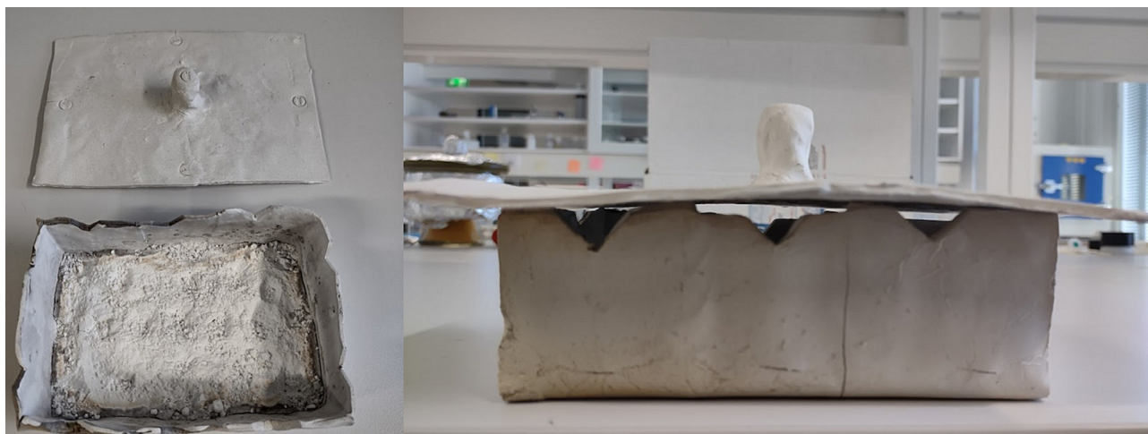
Fig. 3. The container for the 100 g hackmanite batch. Gas flow grooves can be seen in the sides. The container's size is 15 × 10 × 5 cm.
